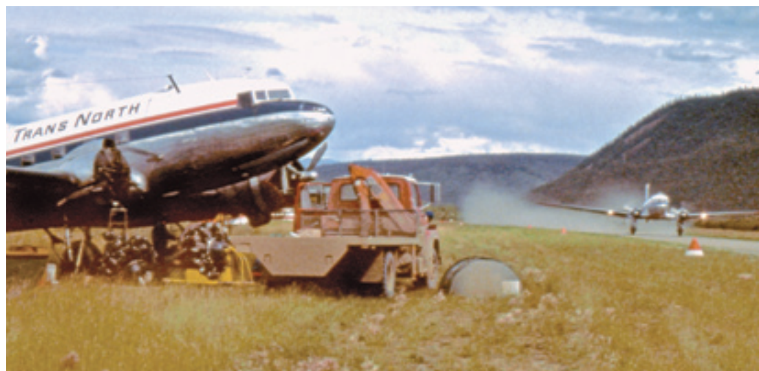
Above: A DC3 engine change beside the runway in Dawson City in the early '80s. In this photo, the failed engine has just been removed while the overhauled engine awaits installation. On the right another DC-3 takes off.
